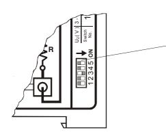
Set the DIP switch to select the secondary voltage range that will be used. With extreme low resistance heatseal elements (less than 100 mOhm) or with extremely high secondary currents (larger than 80 A) additional switch No.5 must be ON.
