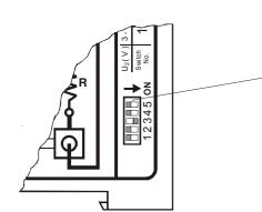
Set the DIP switch to select the secondary voltage range that will be used. With extreme low resistance heatseal elements (less than 100 mOhm) or with extremely high secondary currents (larger than 80 A) additional switch No.5 must be ON.
