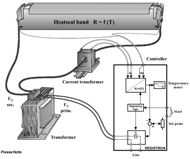
The **RES** temperature controllers are important components for modern machines with higher speeds. The technical possibilities offered by this control system however, can only be achieved by optimizing the complete system. The heatseal element, the heatseal transformer, the wiring, the signaling, and the controller must be perfectly matched for best results.
